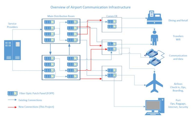
In early 2000's, the port established the Communication Infrastructure Backbone System (CIBS). This created the Main Distribution Rooms (MDR) and the outlying communications equipment rooms (ER).
